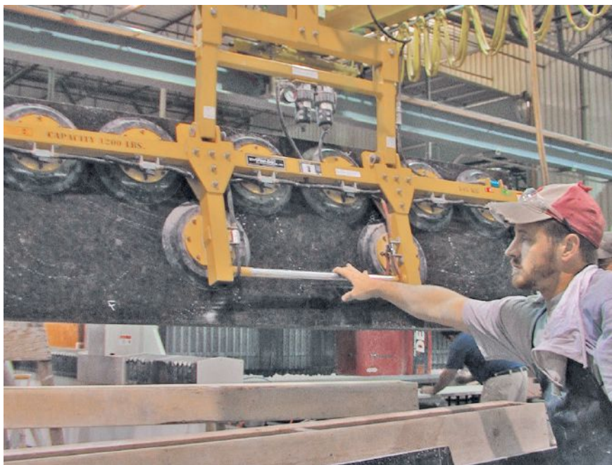
A vacuum lifter is in place to move slabs safely around the workspace.
