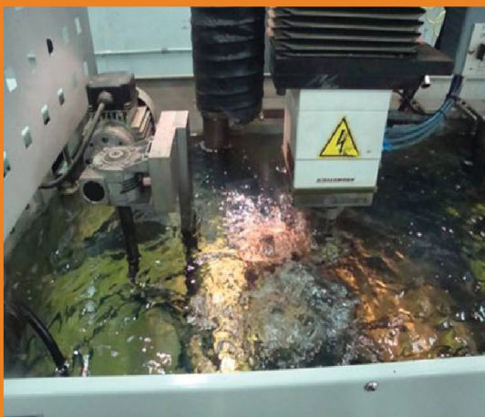
The Electrical Discharge Machining (EDM) process is a critical step in precision re-dressing of CNC tooling.
