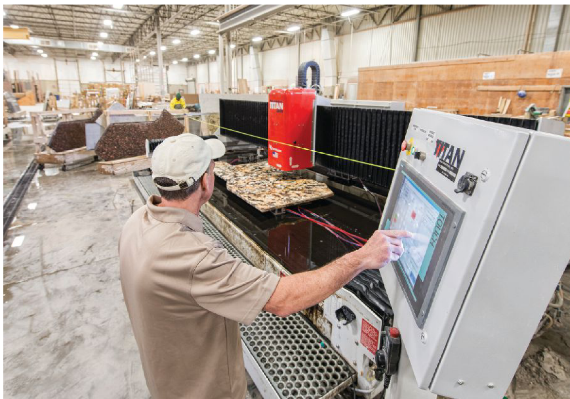
Among the lineup of machinery utilized by Sims-Lohman in the fabrication process is a Titan CNC stoneworking machine from Park Industries of St. Cloud, MN.
