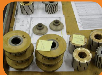
Worn CNC tooling is logged in and prepared for re-dressing.
