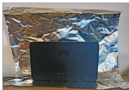
Robert placed foil behind his router to reflect its signal inwards
