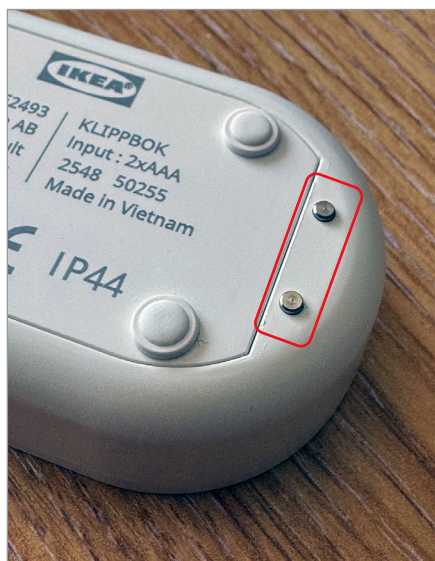
Two metal contacts on the underside of the sensor detect water
