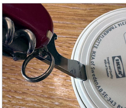
Use a flathead screwdriver to prise the back off the thermometer
