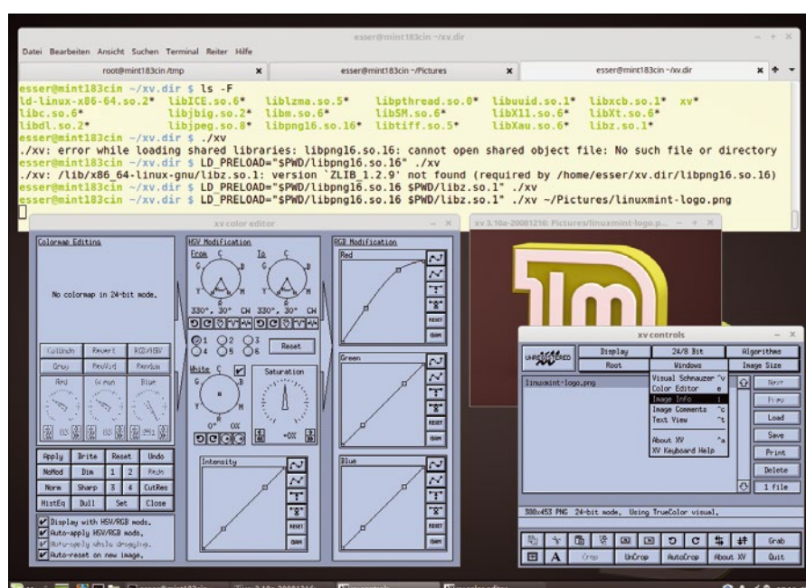
Figure 4: Setting the LD_PRELOAD variables forces the program loader to try the library files that you provide when loading a program.
