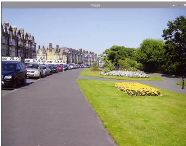
Figure 3: The object recognition elements are shown in the original image along with the percent likelihood of correct recognition.
