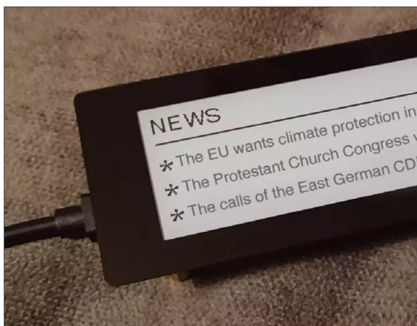
Figure 4: The ePaper display only requires energy when changing the display.
