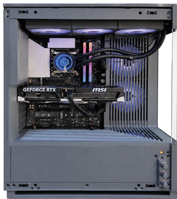
BELOW Angled vents on the inside push cool air towards the core components
