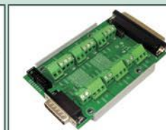
PS12DC Power Switching Board
