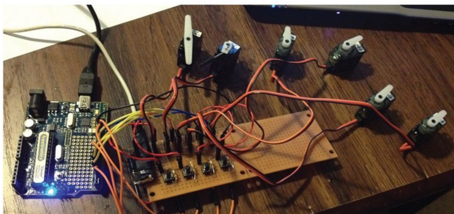
Figure 14. Testing the control board PCB connected to an Arduino Uno, with all six servos.
