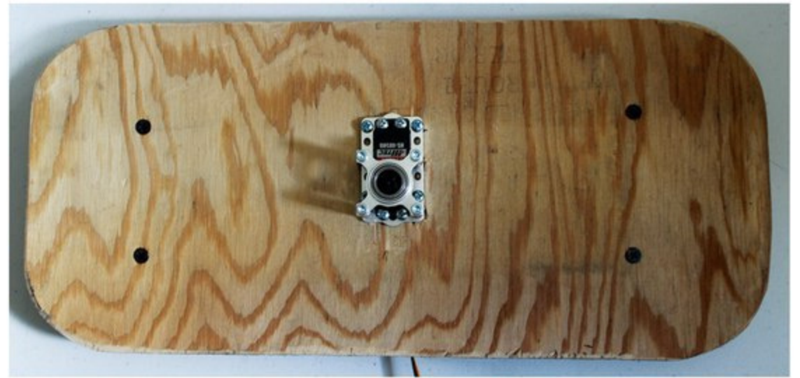
Figure 11. Rotate servo mounted in the shoulder plate.
