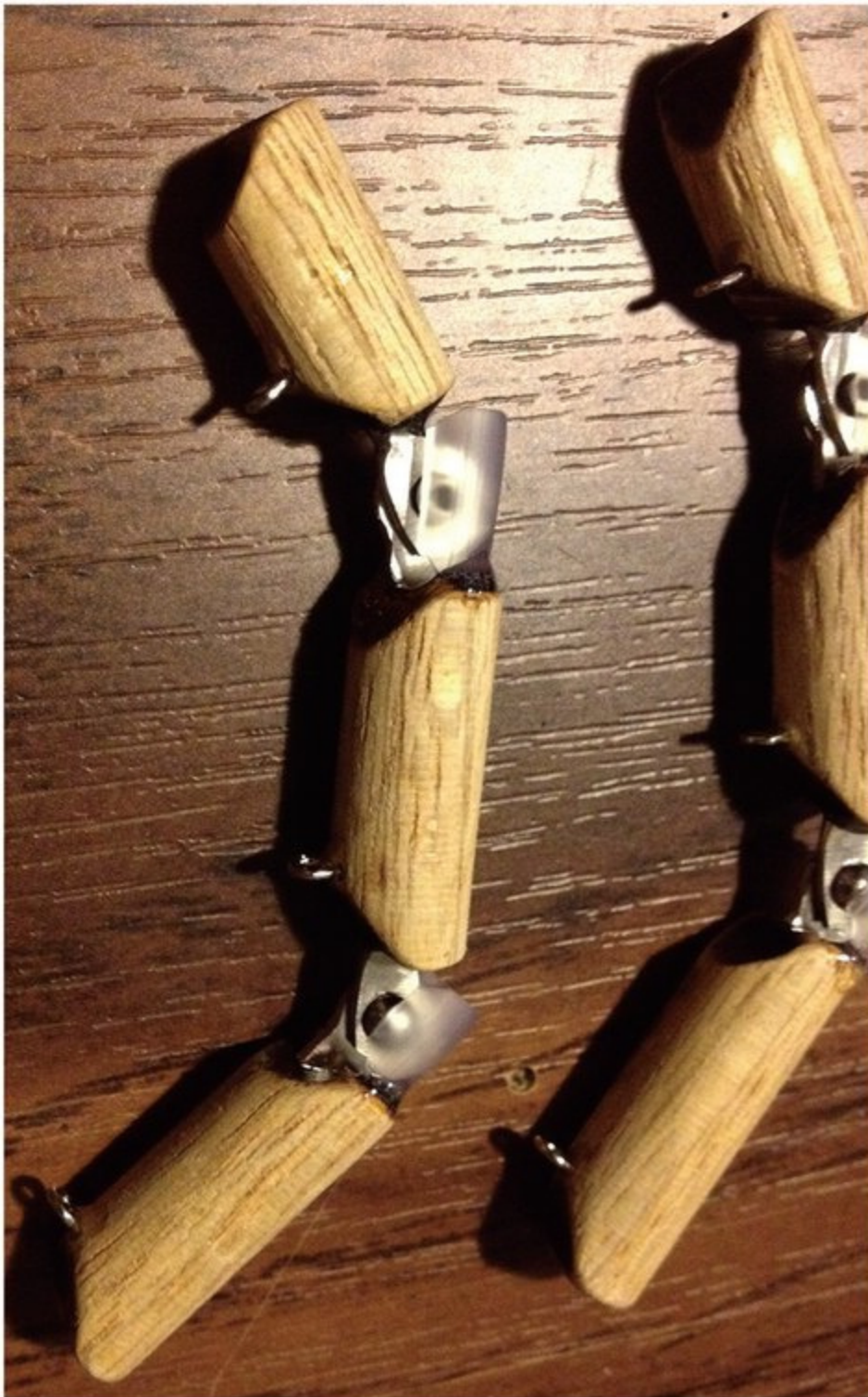
Figure 7. Tendon guides and cartilage cushion/stop added. Tip of finger is at left.
