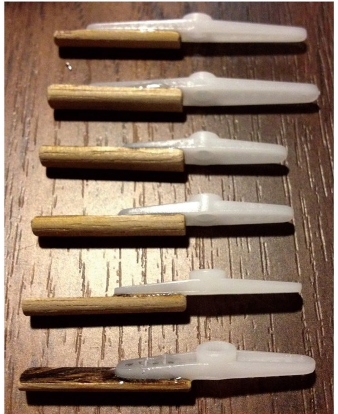
Figure 16. Servo horn extensions — used to increase the servo travel angle horizontal distance — so fingers could be fully closed and opened.
