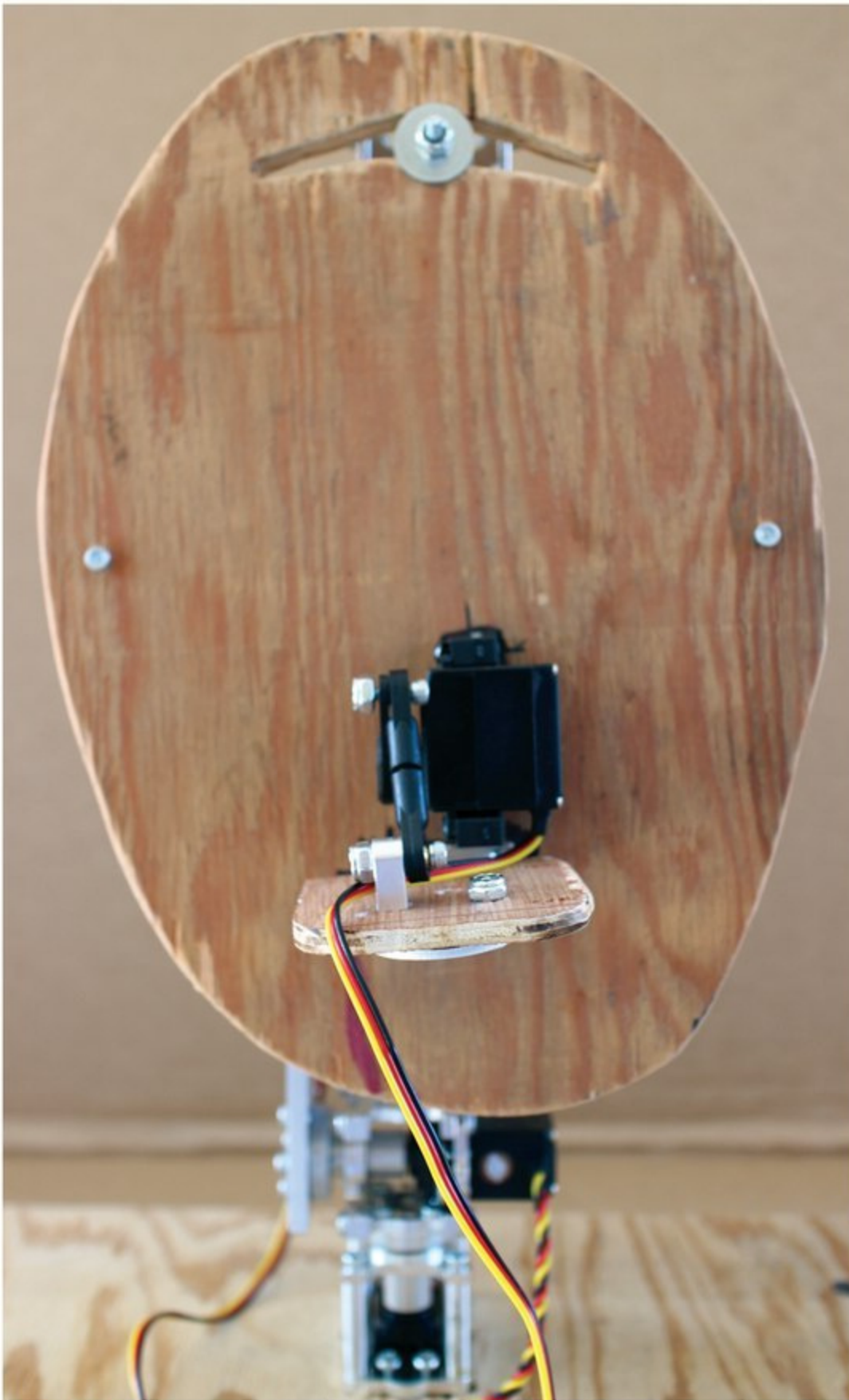
Figure 17. Wood face plate added; just needing some foam.
