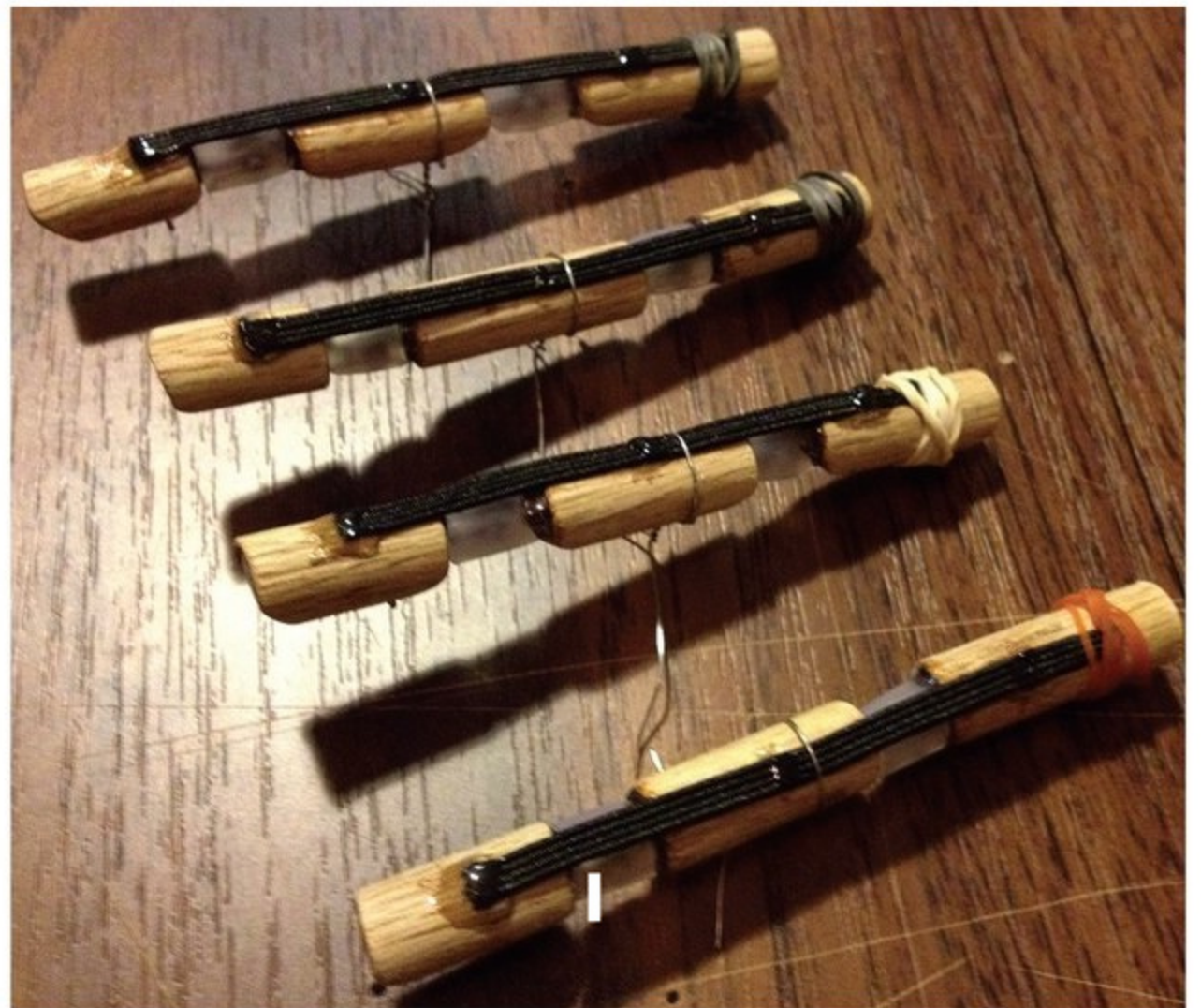
Figure 8. All four fingers with elastic resistance strip applied and curing.
