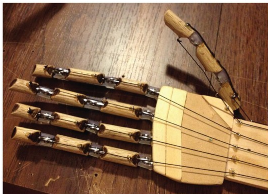
Figure 13. Tendons all threaded and ready. The anchor point to swivel the thumb assembly can be seen at the bottom of the thumb.
