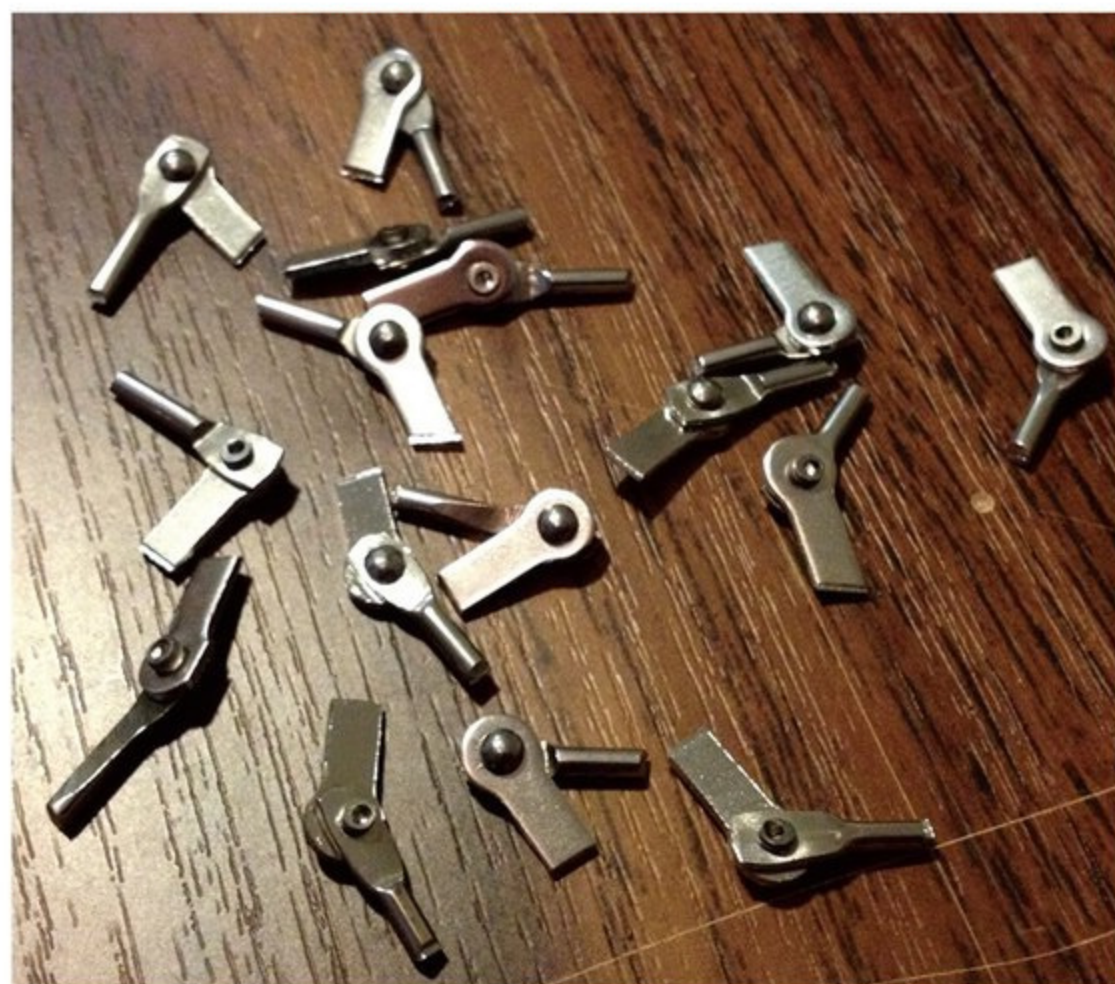
Figure 6. Hinges cut out from tea infusers and ready for use.
