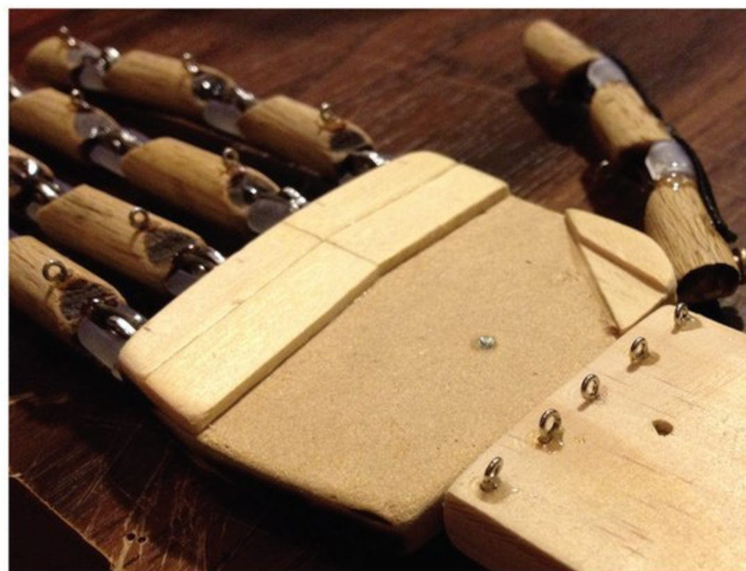
Figure 11. Tendon guides on the forearm for all five digits. Not shown are the eyelets to swing the thumb assembly up.
