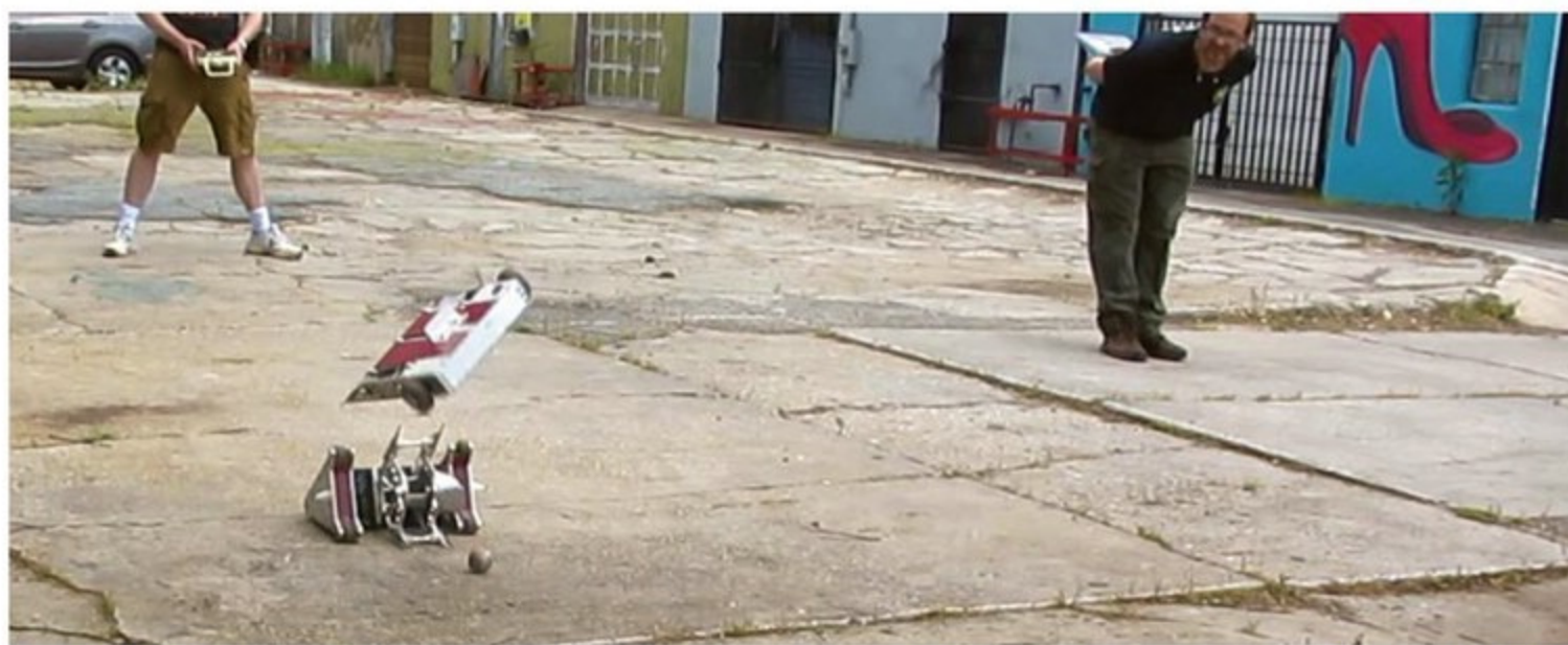
Omega Force launches Abrasive Personality into the air with its kinetic energy flipper.
