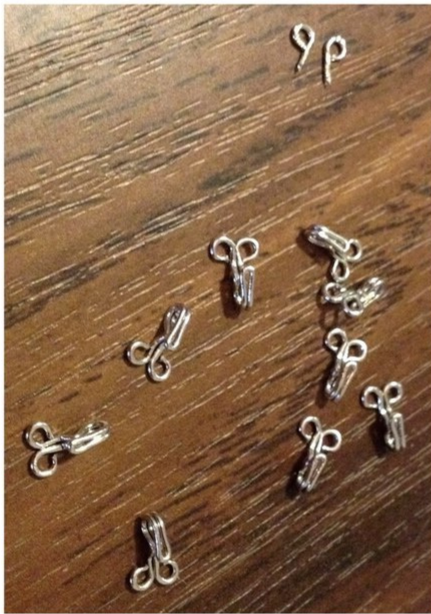
Figure 3. Eyelets to guide tendons. Note the 'cut-and-ready' pair at right.
