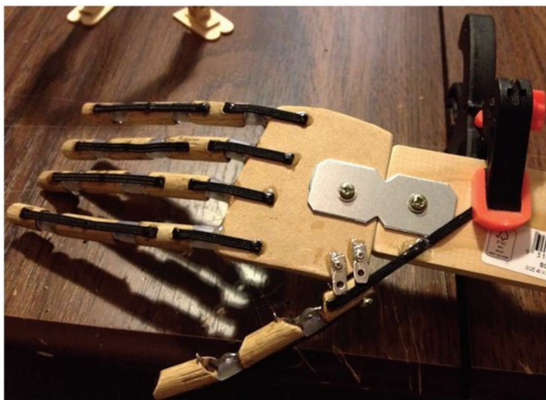
Figure 10. The mechanics are complete. The final step was applying the thumb assembly return elastic.
