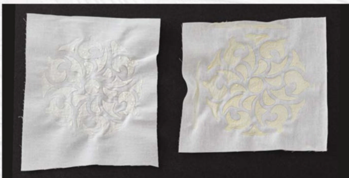
Samples of potato dextrin (left) and corn dextrin applied to fabric through a stencil.
