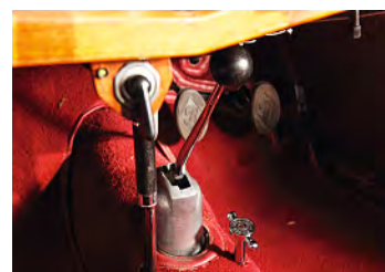
Double-declutching is essential on all Nines, bar those with overdrive or preselector 'boxes; knob alongside is for cable adjustment (on cable-brake cars)
