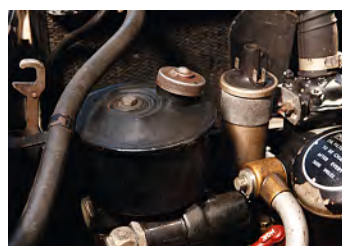
Power steering is desirable on S1s, and later standard. Ponderous due to its many turns lock-lock, but something's worn if there is significant free play
