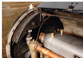
Radiators were always nickel-plated on the 3 Litres; corrosion means a costly rebuild. Pre-chassis 1003 cars had no header tank; 1092-on were 1in taller
