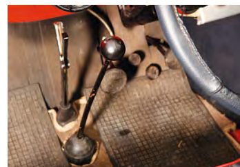
Ford had more ball- and roller-bearings than any rival; five were in the gearbox, but it will wear out. Multi-plate clutch ('28 only) best replaced by single-plate
