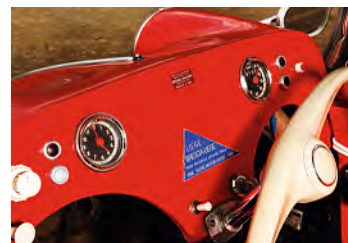
Spartan dash is well equipped with warning lights, such as for electrically selected reverse; it runs the engine backwards to give four reverse gears
