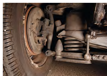
Maintenance is key to long suspension life - look out for recent lubrication. Inspect the rear dampers for leaks; they can be reconditioned for c£100 each
