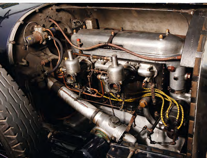
An engine rebuild is expensive: establish its health and adjust the price accordingly. Expect 15-20psi oil pressure on a run - less means wear or internal bleeding. Ask to see bills for past engine work. A Phoenix counterbalanced crank is good and usually means shell bearings, which tolerate modern oils - otherwise, using SAE50 is best
