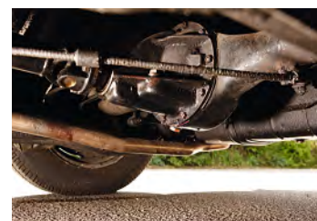
Crownwheel carrier is prone to cracks, exacerbated by rough gearshifts: best to match revs when changing down. A rebuild can be £2k+ including parts
