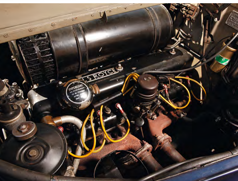
Look for signs of regular maintenance on both engines. Correct antifreeze is key, as are oil changes: inspect for signs of overheating, plus water/oil leaks. These durable engines do wear out and are costly to rebuild (a secondhand 'six' is c£7800). HD6 carbs on the 'six' and early V8s give better economy, HD8s better performance
