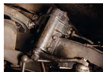
The steering ratio was progressively tightened during production; early cars can be updated to a later spec. A worn steering box can be rebuilt for c£400
