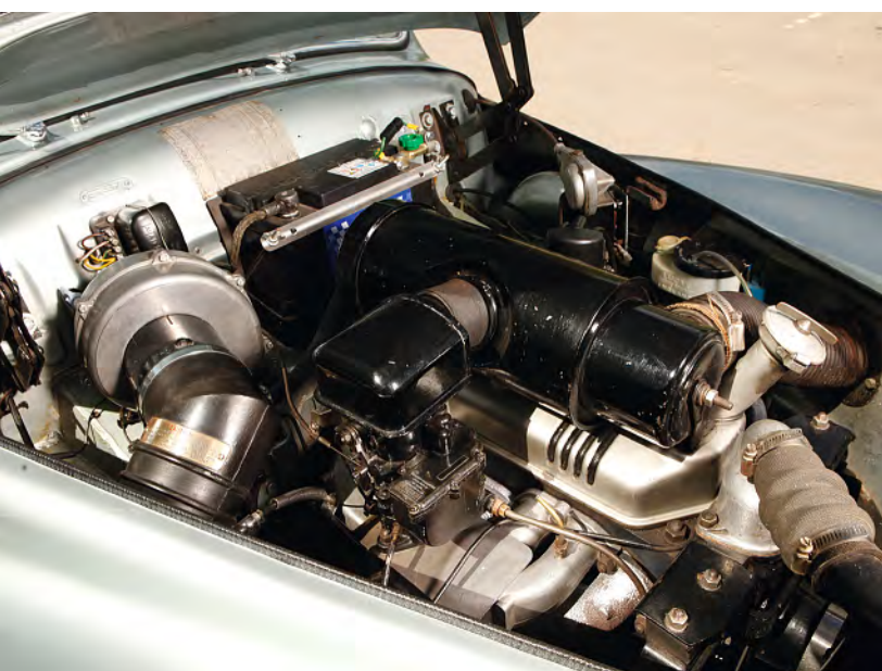
Engines are simple, sturdy and long-lived if regularly serviced, but oil leaks can be an issue. Seven-port heads (on all cars pre-MkIII/Alpine) are liable to crack around cylinders two and three, into the exhaust valve seats; check for poor running and/or overheating or water loss. The eight-port (as here, check inlet manifold) is stronger
