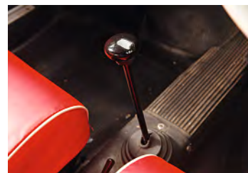
The gearchange was highly rated when new and should still feel smooth, with synchro on the upper three ratios. It is robust and can handle uprated engines
