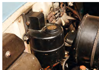
S1s have a pedal-operated oil-lubrication system: it's prone to blockage when old, leading to rapid suspension wear. Later cars require annual lubrication
