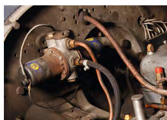
A vacuum-powered Autovac fuel pump was standard, but proved inadequate on long inclines: this double-ended SU electric pump is the ideal alternative
