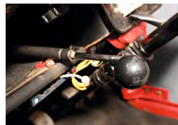
The unconventional dog-leg gearchange should be easy and crunch-free. Test the synchromesh (especially in third) and listen for noise from worn bearings
