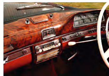
All six-cylinder cars had wood interior trim on the dash and door cappings. If the former needs to be restored or changed, it is a windscreen-out job
