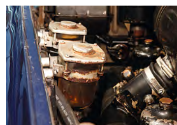
Among the best drums around, Cloud brakes will seize if left unused for long periods. The servo (a Hispano-Suiza design) requires specialist maintenance
