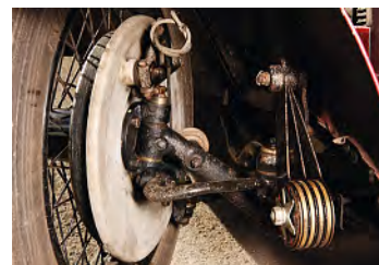
All parts can be found to rebuild worn front suspension, but it can cost £3000 if it needs new stub-axles and kingpins, so frequent lubrication is sensible
