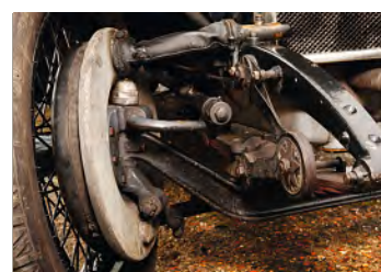
All suspension points should be oiled every six months or 2000 miles. Worn bearings and shackle pins mean heavy steering, and can affect the handling
