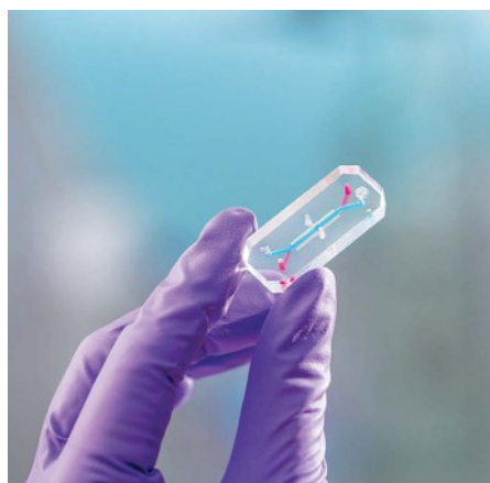
The AVATAR experiment carried several USB drive-sized organ chips, containing bone marrow cells derived from each astronaut’s blood, along for the 10-day spaceflight. Once on the ground, the chips were transferred to laboratories for analysis of the effects of space travel on the cells. EMULATE/NASA
