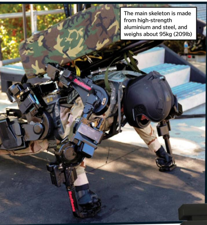
The main skeleton is made from high-strength aluminium and steel, and weighs about 95kg (209lb)
