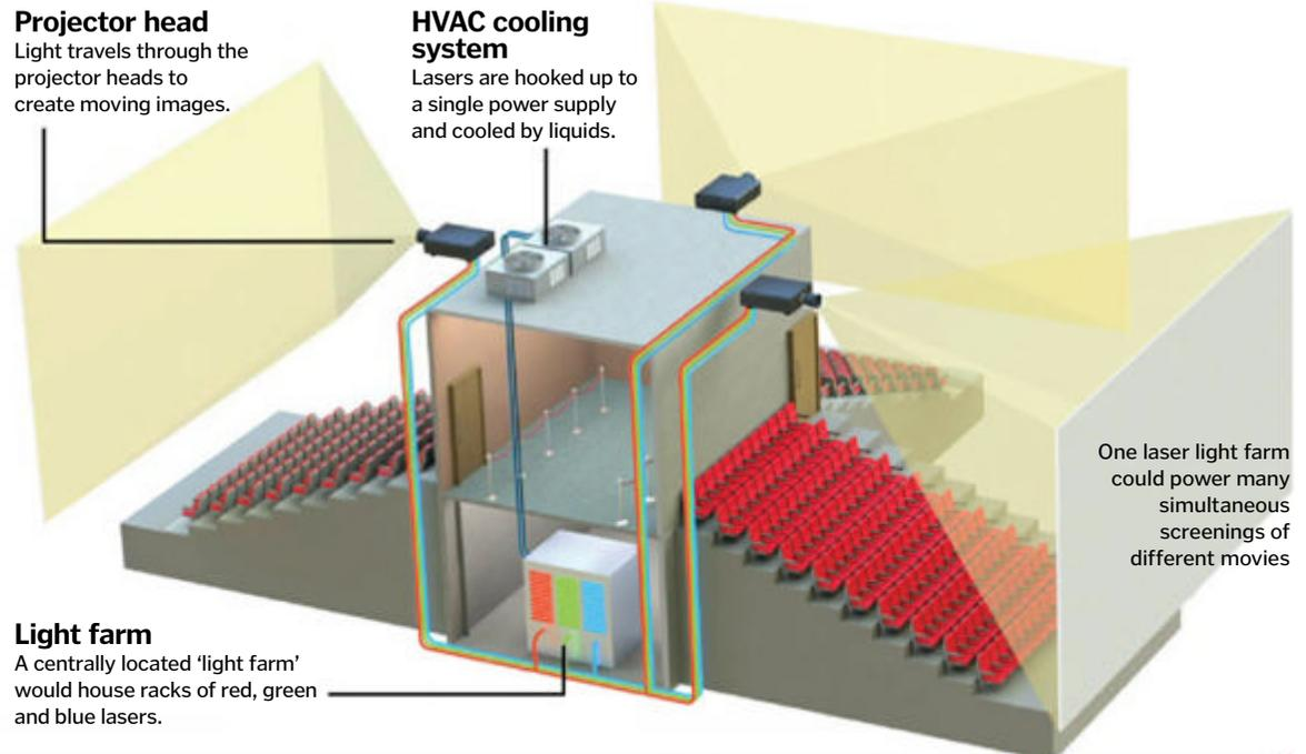
One laser light farm could power many simultaneous screenings of different movies
