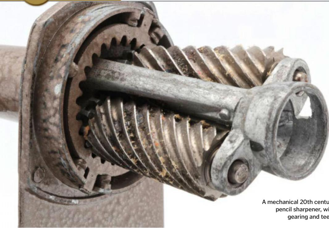
A mechanical 20th century pencil sharpener, with gearing and teeth
