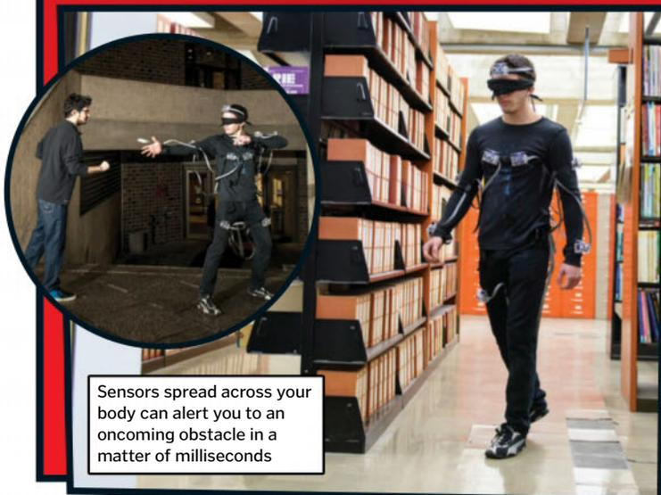
Sensors spread across your body can alert you to an oncoming obstacle in a matter of milliseconds
