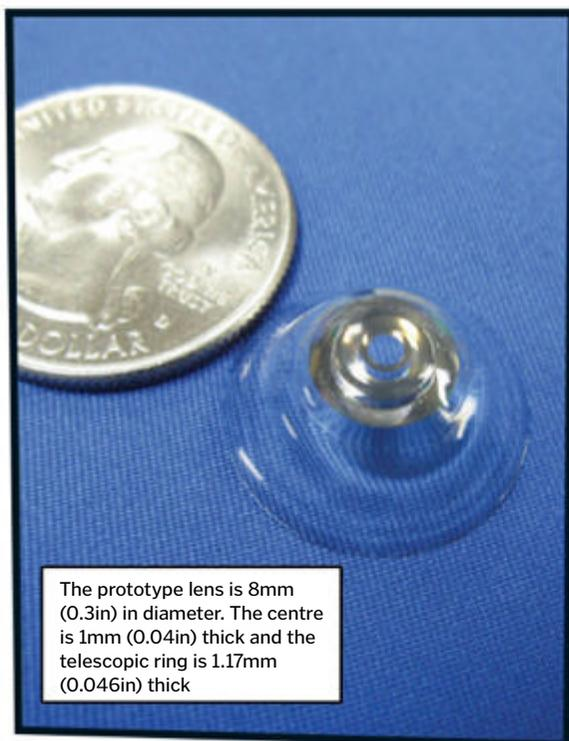
The prototype lens is 8mm (0.3in) in diameter. The centre is 1mm (0.04in) thick and the telescopic ring is 1.17mm (0.046in) thick
