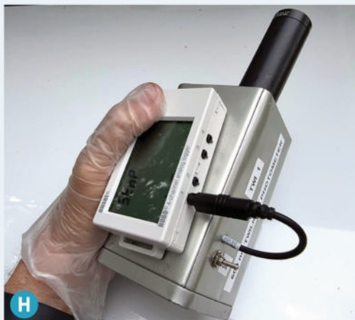
H Completed twilight photometer.
