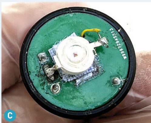
Lower side of circuit board showing the LED. Note that the LED anode is soldered to the junction of two center tabs from the socket on the front side of the board.
