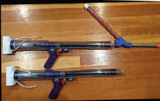
THE LATE RYAN "MCNUMBERS" KRETERFIELD OF MOSTLY HARMLESS ARMS BUILT THE BEST DIY BLASTER OF ITS DAY, THE RAINBOWPUMP, USING PVC PIPE AND OFF-THE-SHELF HARDWARE FROM McMaster-Carr.
