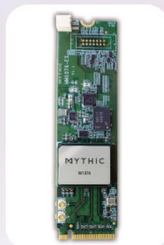
Well-funded startups like Mythic are already building analog chips for AI, promising to vastly reduce energy needs.
