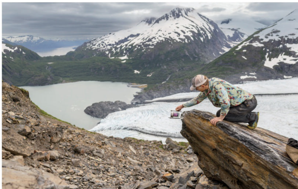
Hig’s $300 radar instrument, housed in a mason jar, bounces a signal off a nearby reflector plate to continuously monitor landslide movement. The sensor then transmits its data wirelessly.
