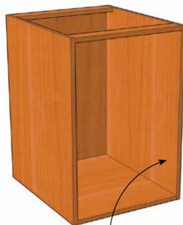
FRAMELESS Hinges mount to the cabinet interior.
